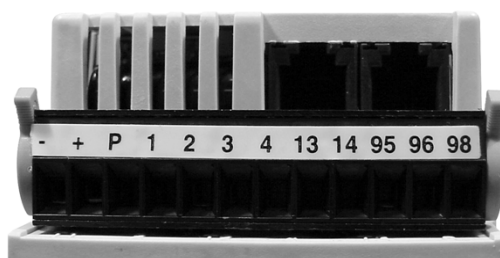
Figure 3-9: Terminal Block
