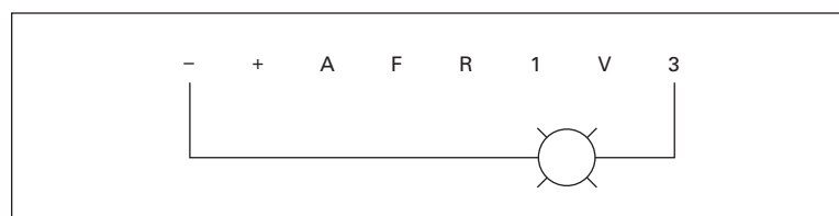
Figure 16: Alarm Output Wiring
